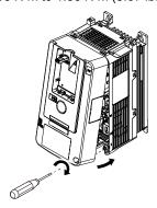
Figure 8.8 Install the Front Cover
